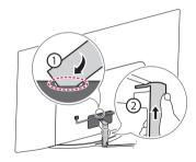
Do not use a sharp object when you detached the cable cover. This could damage the cable or the cabinet. It may also cause personal harm, (Depending upon model).
